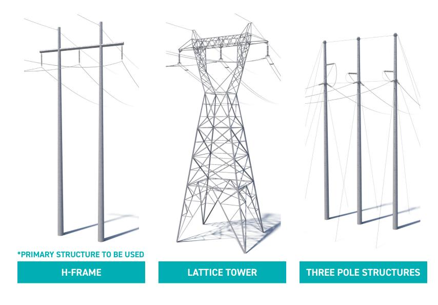
Crews plan to install steel H-frame, lattice tower and three-pole structures along the line route
